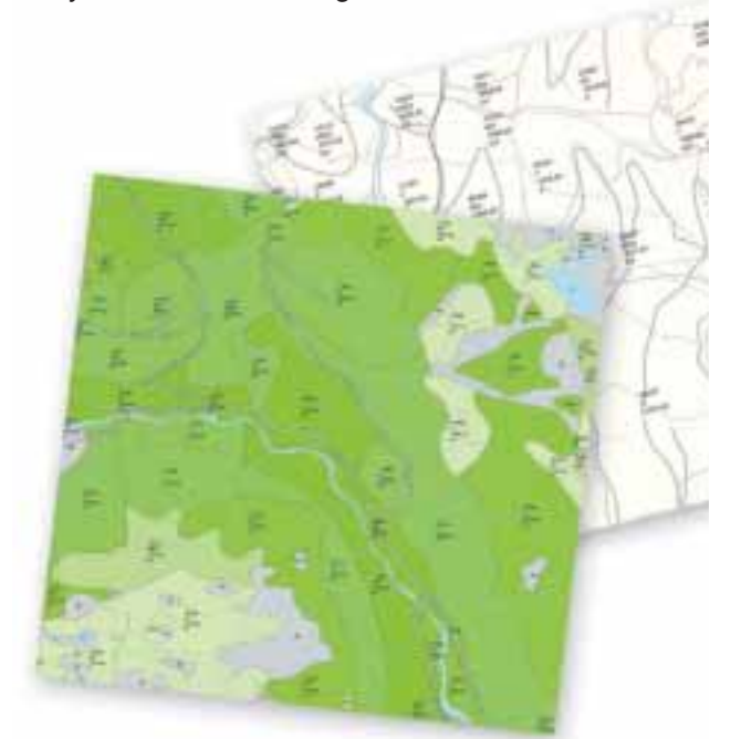
▲ Inventory data is used to create computer-generated forest cover maps (above right) that identify stands of different species, ages and heights. A similar area (left) is classified by stand productivity.
